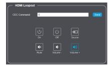
Send user-defined or preset CEC commands to HDMI IN and HDMI Loop-out.
