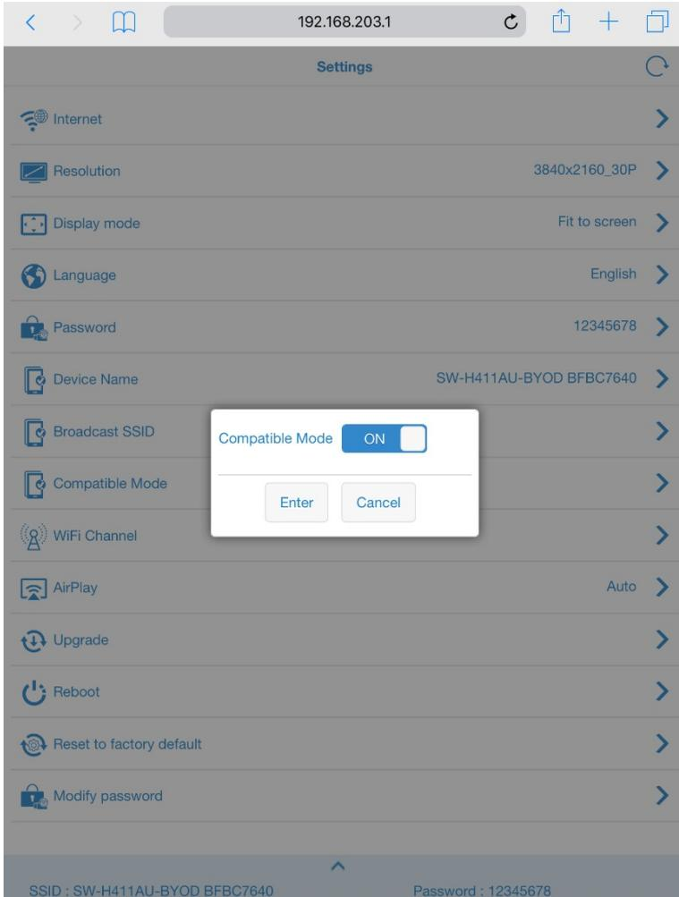
When select "ON", the system is compatible with more wireless source devices.
