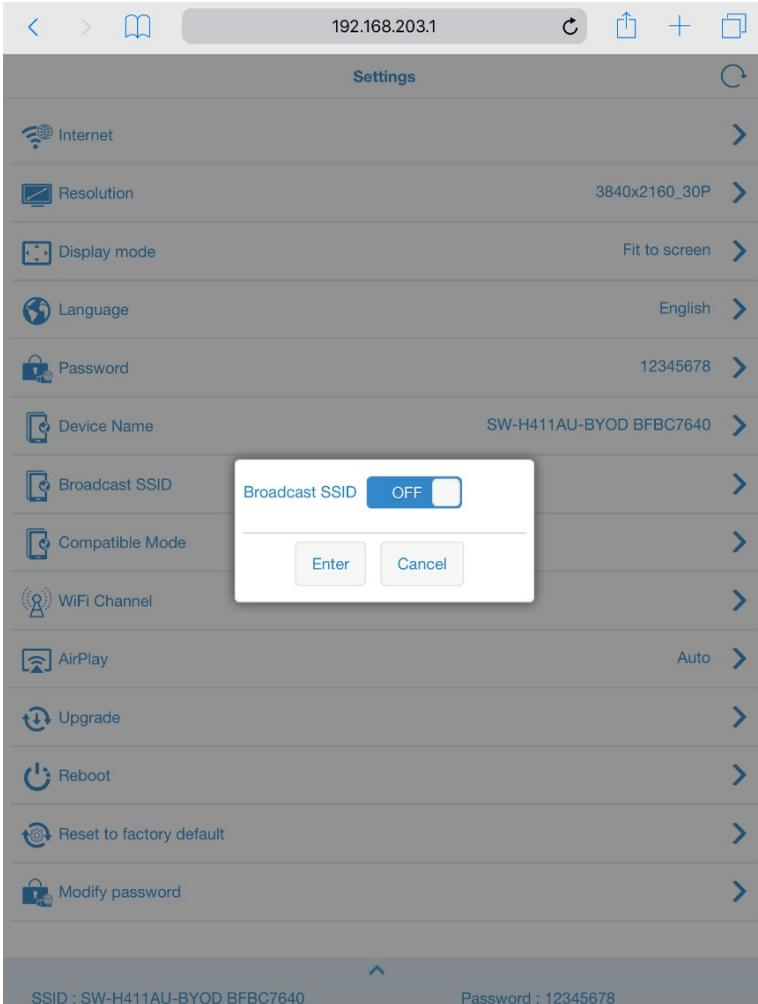
When select “OFF”, the SSID will not be found by wireless source device, but it can be connected by manually adding a new network.
